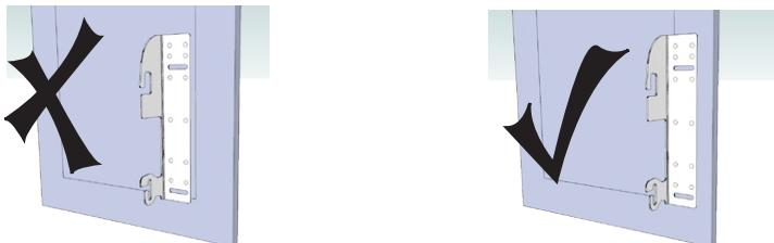
The door brackets should line up with the thick portion of the cabinet door.
